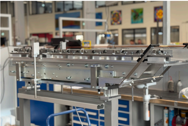
Typical application: SLL 800-1200 as accumulation section
