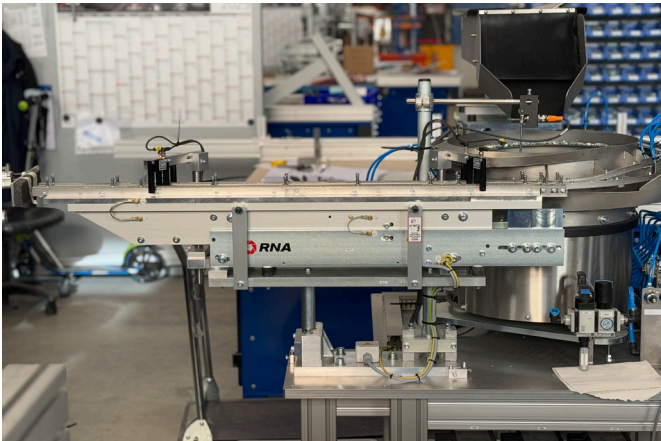
Typical application: SLL 804 as accumulation and feeding section
